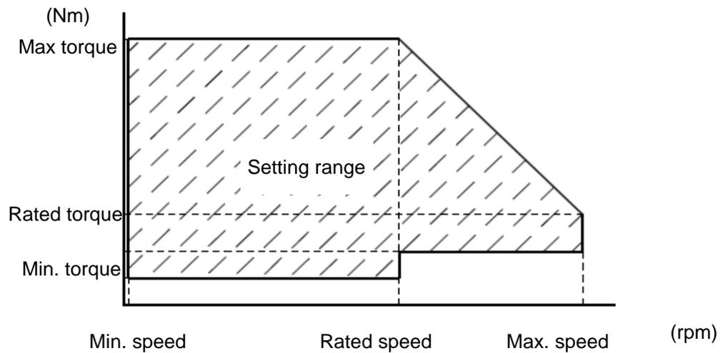
Output speed and torque is set to the indicated value.
